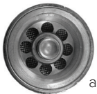
a clear valve no blockage
